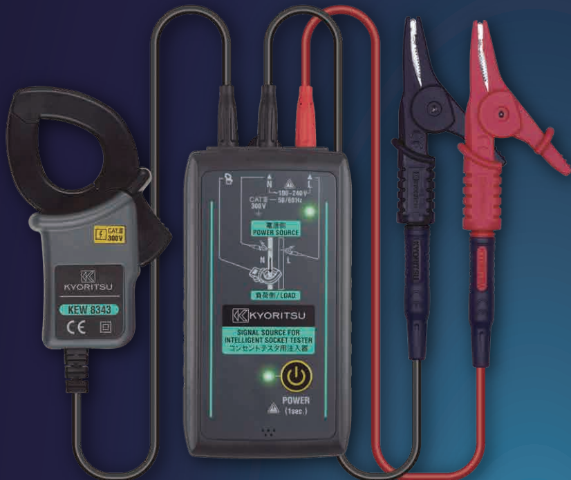
SIGNAL SOURCE FOR INTELLIGENT SOCKET TESTER KEW 8343
