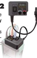
For taking single phase supply (100-240V) from the test leads to power the instrument (FUSE: 8923)
